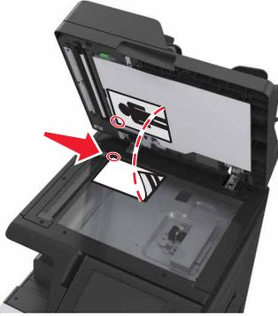
An illustration of a scanner's glass with a document placed on it. Red arrows point to the corners of the document. <ul style="list-style-type: none"><li>• 扫描仪玻璃用于单页文档、书页、小物品（如明信片或照片）、透明胶片、照片纸或薄介质（如杂志剪报）。</li><li>• 将文档面朝下放在有箭头的角落中。</li></ul> |
